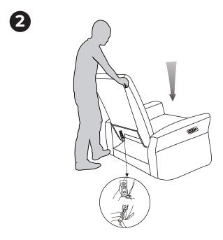
Slide the Backrest into the metallic quick connectors of the Seat. Push down the Backrest firmly until each side is locked into place and an audible "click" is heard.
