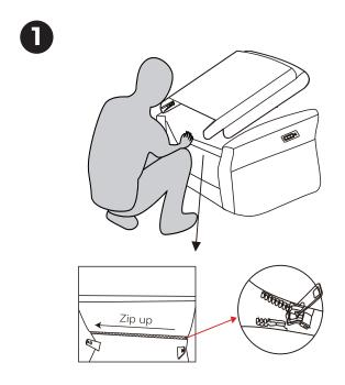
Zip up the bottom of the back and the seat together.
