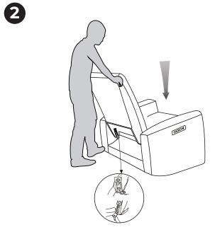
Slide the Backrest into the metallic quick connectors of the Seat. Push down the Backrest firmly until each side is locked into place and an audible "click" is heard.
