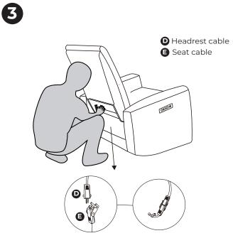
Connect the cable D into cable E.
