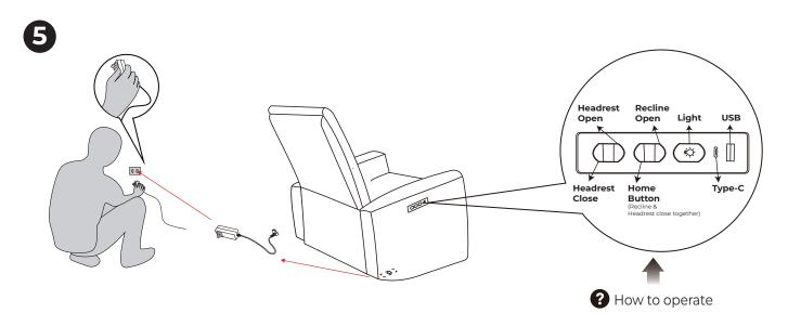
Connect one end of the power cord into the DC adaptor located at the bottom corner of the seat. Plug the other end of power cord into the power outlet.
