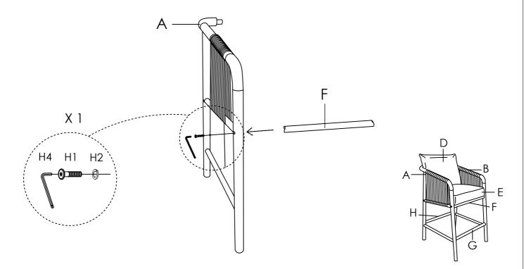
Assemble the Backrest (C) using Lock Washers (H2), Short Bolts (H1) and Allen Wrench (H4). **Do not fully tighten yet.**
