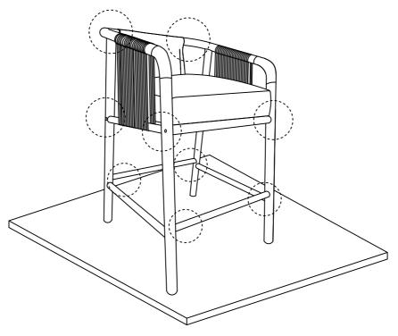
Gently tap the Wooden Plugs (H8) into Left Arm and Right Arm. Put on the Back Cushion (D). Assembly complete.
