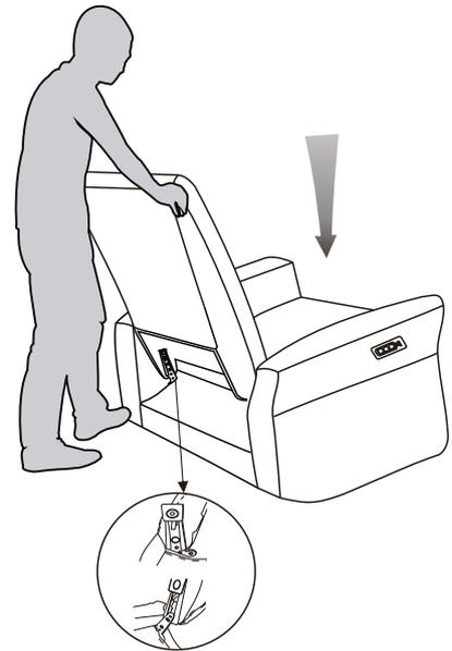
Slide the Backrest into the metallic quick connectors of the Seat. Push down the Backrest firmly until each side is locked into place and an audible “click” is heard.
