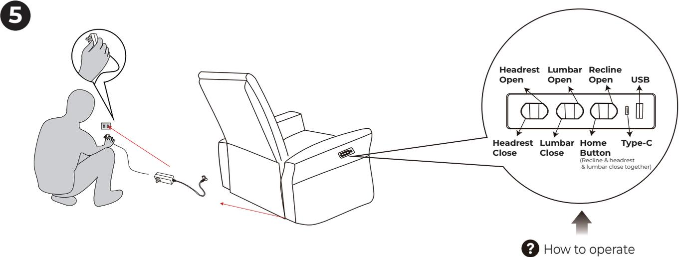
Connect one end of the power cord into the DC adaptor located at the back corner of the seat. Plug the other end of power cord into the power outlet. Note: After all the connections are made, the green LED will be lit up.
