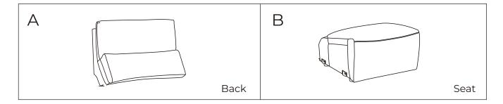
Step 1: Slide the Back (A) into the metallic quick connectors of the Seat (B). Push down the Back (A) firmly until each side is locked into place and an audible "click" is heard.
