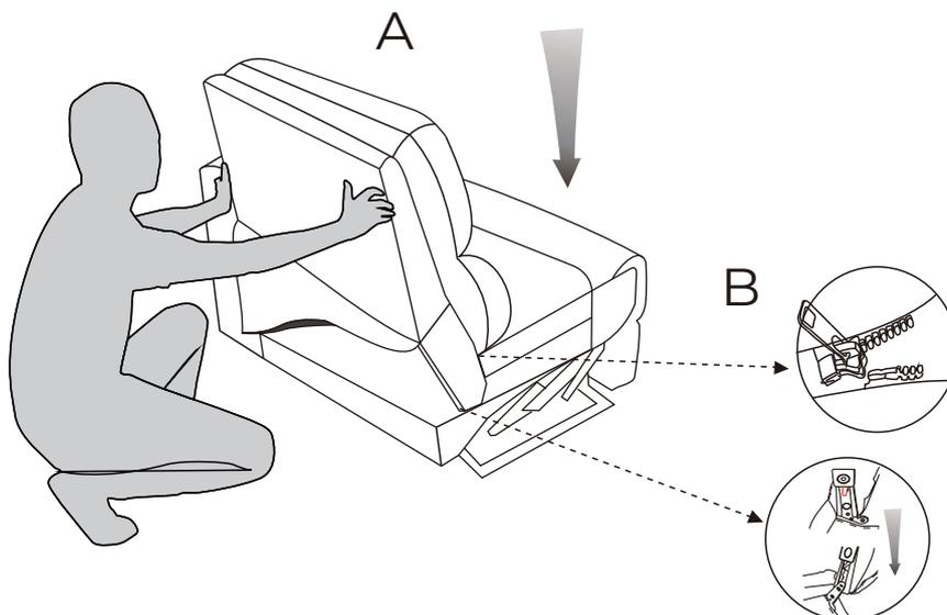
**Step 2: Connect the cable D into cable E.**
