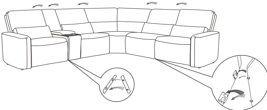
**Step 2: Connect the wire piece by piece.**
