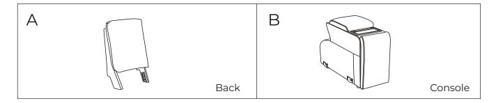
Step 1: Slide the Back (A) into the metallic quick connectors of the Console (B). Push down the Back (A) firmly until each side is locked into place and an audible "click" is heard.
