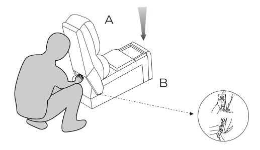
Step 2: Attach the back cover to the bottom of the Console (B) with Velcro.
