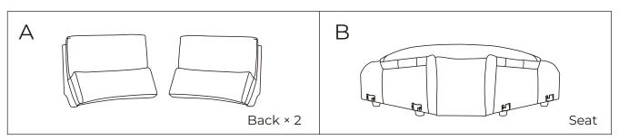
Step 1: Slide both Backs (A) one after the other into the metallic quick connectors of the Seat (B). Push down both Backs (A) firmly until each side is locked into place and an audible "click" is heard.
