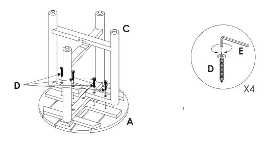
3 Turn assembled side table upright and place on a flat surface. Push legs up or down as necessary to level. Once level, tighten all screws.
