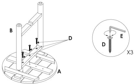
2 Use an Allen Wrench (E) to tighten the Screw (D) on the Leg Frame (C) to the Table Top (A). Do not fully tighten them yet.
