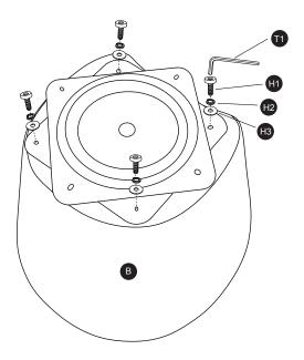
Attach the Chair Base (B) to the Chair Body (A) using Bolts (H1), Spring Washers (H2), and Flat Washers (H3). First, rotate the Chair Base (B) by 45 degrees and loosely attach the first bolt. Then sequentially turn by 45 degrees to attach the remaining bolts.
