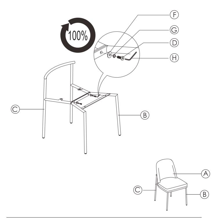
2 Attach the Seat & Back (A) to the assembled chair frame from Step 1, using Flat Washers (F), Spring Washers (G), Long Bolts (E), and Allen Wrench (H). Fully tighten.
