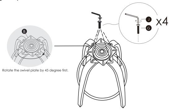
4 Put the assembled stool base in Step 3 on a flat surface. Push legs left or right as necessary to level. Once level, **fully tighten all bolts.**
