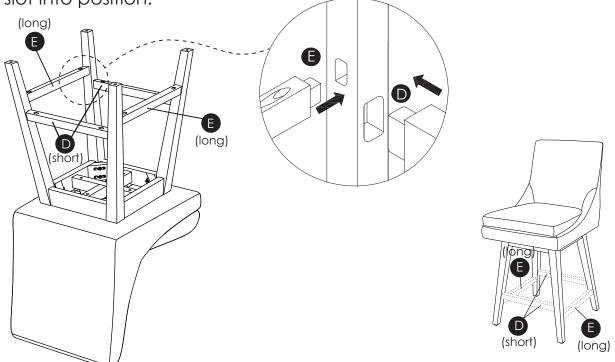
3 Attach the rails using screws (H1). Do NOT start the screws if the rails are not fully slotted into position.
