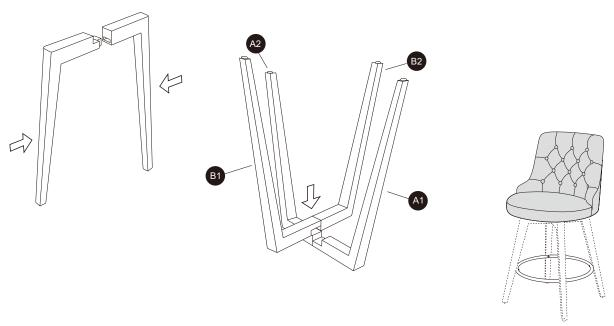
Plip over the stool base. Loosely attach the Bolts (H2) one by one and keep them loose. Do not fully tighten. After loosely attach the first bolt, move on to the diagonal bolt. After all 4 bolts are attached, use Allen Wrench (T1) to tighten.
