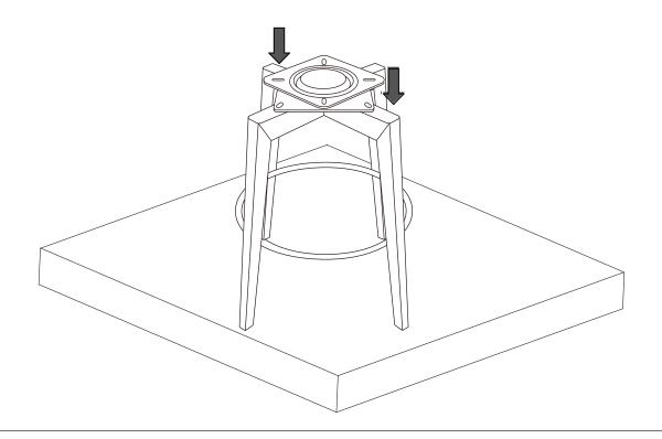
5 Attach the assembled stool base in Step 4 to the Seat Bucket (C), using Shortest Bolts (H3), Lock Washers (H4), Flat Washers (H5) and Allen Wrench (T1). Fully tighten all bolts.
