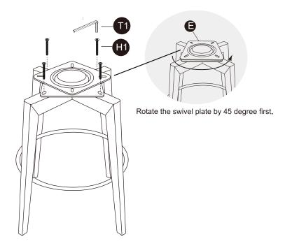
Put assembled stool base in Step 3 on a flat surface. Push legs up or down as necessary to level. Once level, fully tighten all bolts.
