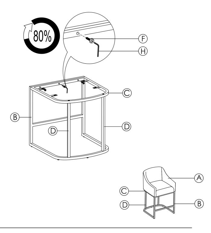
4 Use Allen Wrench (H) to fully tighten all bolts in Step 1, 2, and 3 (seven bolts in total).
