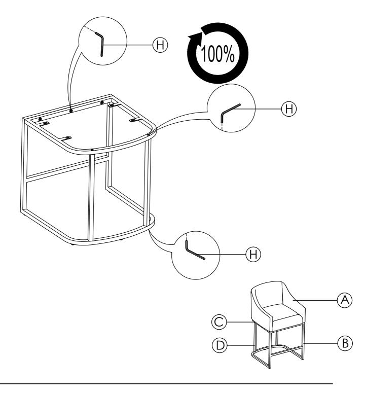
**5** Attach the Seat & Back (A) to the assembled stool base from Step 4, using Short Bolts (G) and Allen Wrench (H). **Fully tighten.**
