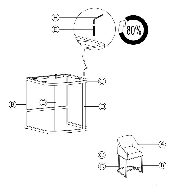
Attach the Top Frame (C) to the Front Leg Frame (B), using Bolts (F) and Allen Wrench (H). **Do not fully tighten yet.**
