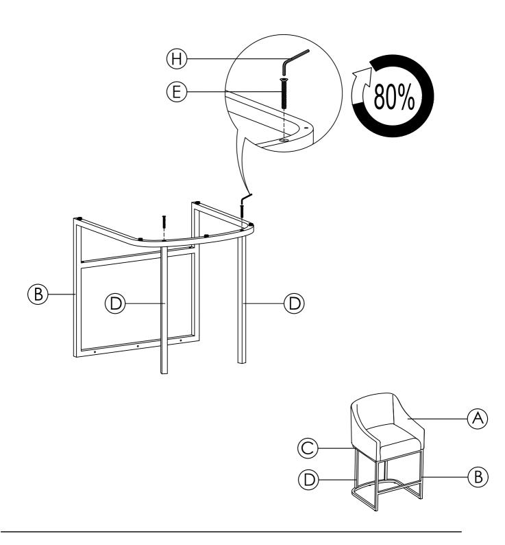
Attach the Top Frame (C) to the Back Legs (D), using Long Bolts (E) and Allen Wrench (H). **Do not fully tighten yet.**
