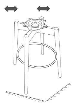
Attach the assembled stool base in Step 4 to the Seat (A), using Short Bolts (G) and Allen Wrench (K). Fully Tighten all bolts.
