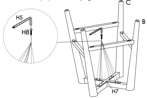
Flip over the stool base. Fully tighten the stool base, using Long Bolt (H1) and Allen Wrench (H5).
