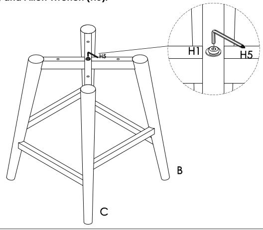
**5** Attach the Swivel Plate (F) to the assembled stool base, using Big Flat Washers (H3), Lock Washers (H2), Long Bolts (H1), and Allen Wrench (H5). **Do not fully tighten.**
