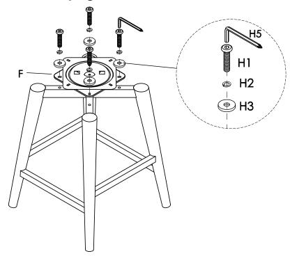
6 Put the assembled stool base on a flat surface. Push legs up or down as necessary to level. Once level, fully tighten all bolts and screws.
