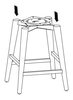
Lean down the stool on the ground and attach the assembled stool base and Seat (A), using Big Flat Washers (H3), Lock Washers (H2), Long Bolts (H1), and Allen Wrench (H5). Fully tighten.
