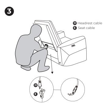
Connect the cable D into cable E.
