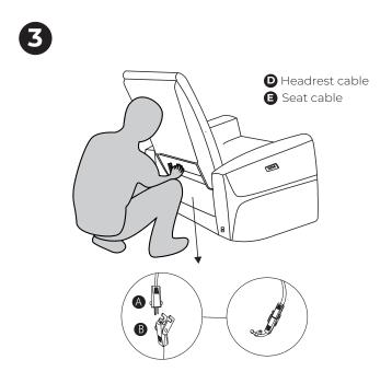
Connect the cable D into cable E.
