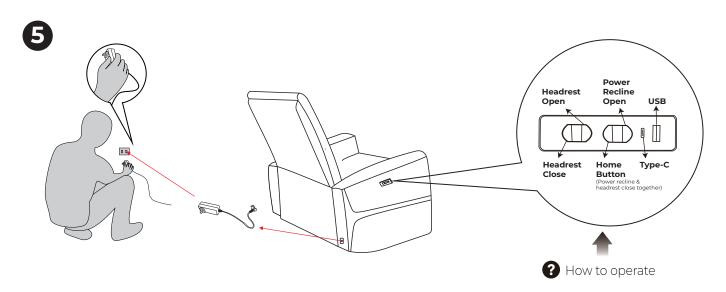
Connect one end of the power cord into the DC adaptor located at the back corner of the seat. Plug the other end of power cord into the power outlet. Note: After all the connections are made, the green LED will be lit up.
