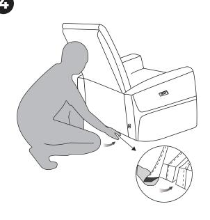
Attach the back cover to the bottom of the seat with Velcro.
