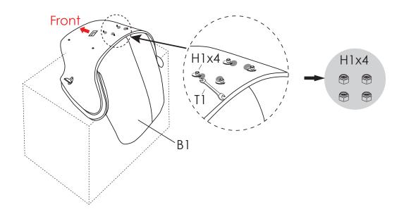
2 Attach the Chair Base (A1) to the Chair Body (B1) using Locknuts (H1) from Step 1 and Wrench (T1).
