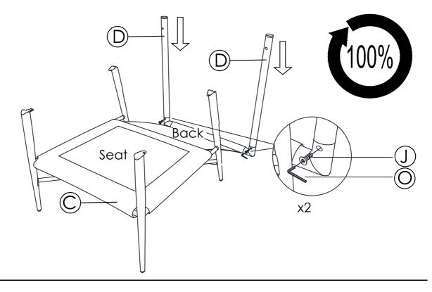
Attach Wood Arms (D) to front legs and back legs, using Bolts (J) and Allen Wrench (O). Start with bolts at the front legs and then move on to the bolts at the back legs. **Do not fully tighten yet.**
