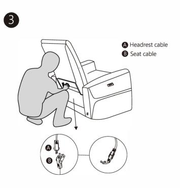
Connect the cable A into cable B.
