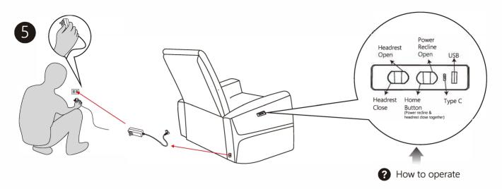
Connect one end of the power cord into the DC adaptor located at the back corner of the seat. Plug the other end of power cord into the power outlet.
