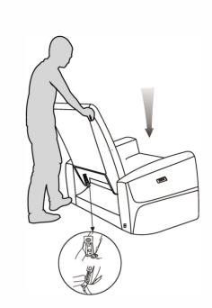
Slide the back into the metallic quick connectors of the base. Push down the back firmly until each side is locked into place and an audible "Click" is heard.
