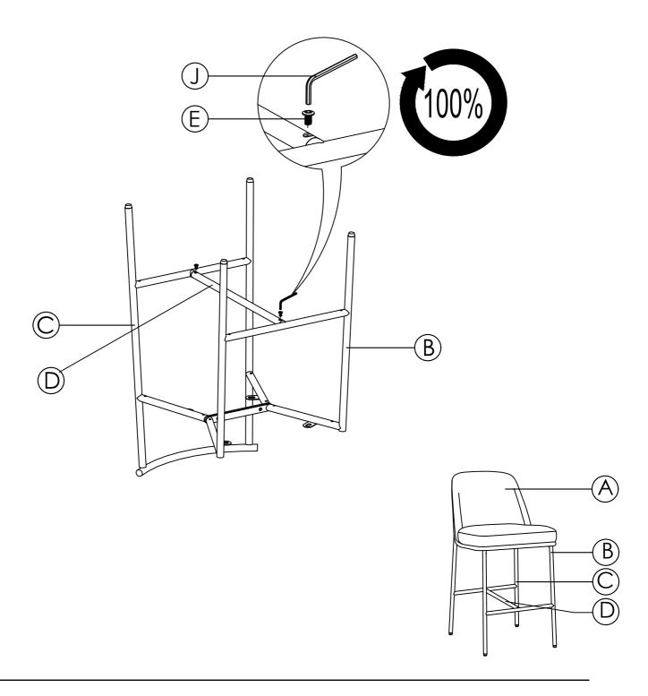
2 Connect Front Leg (B) and Back Leg (C) as indicated below, using Bolts (F), Spring Washers (I), Flat Washers (H), and Allen Wrench (J). Fully tighten.
