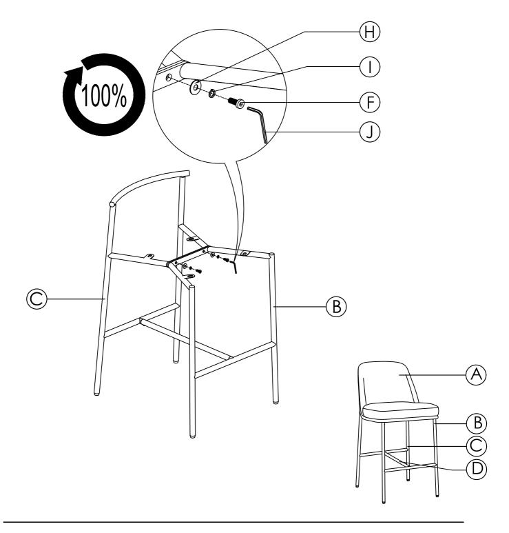
Attach Seat & Back (A) to assembled chair frame from Step 2, using Bolts (G), Spring Washers (I), Flat Washers (H), and Allen Wrench (J). Fully tighten.
