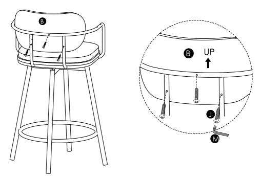
6 Attach Handrail (F) to metal arm using Bolts (J) and Allen Wrench (M).
