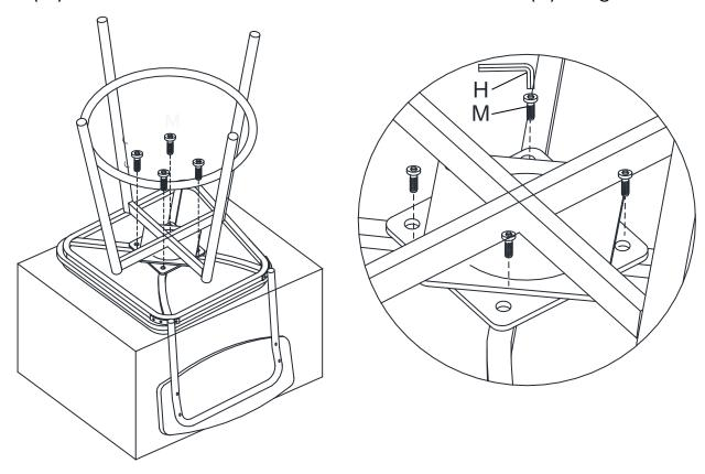
Put assembled stool on a flat surface. Push legs up or down as necessary to level. Once level, tighten all bolts.
