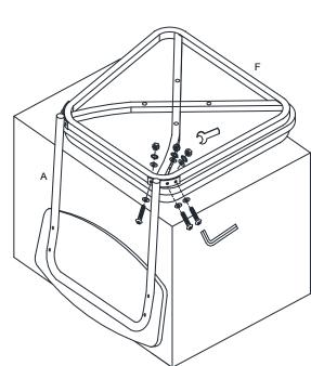
Attach assembled stool base in Step 2 to assembled seat in Step 3, using Bolts (M). After all 4 bolts are attached, use Allen Wrench (H) to tighten.
