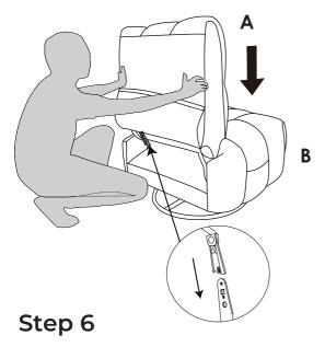
Locate the Power Adapter (E) and connect to its corresponding receiver on base of the Seat (B). Connect one end of the Power Cord for Adapter (D) into the Power Adapter (E).
