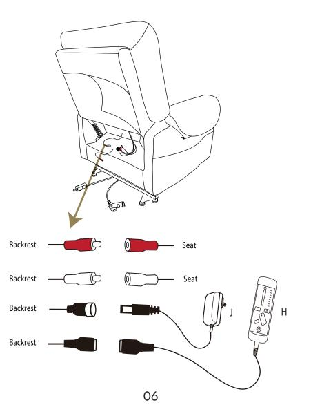
Locate the Remote Control for Lifting & Reclining (G) and connect to its corresponding receiver on the base of the seat.
