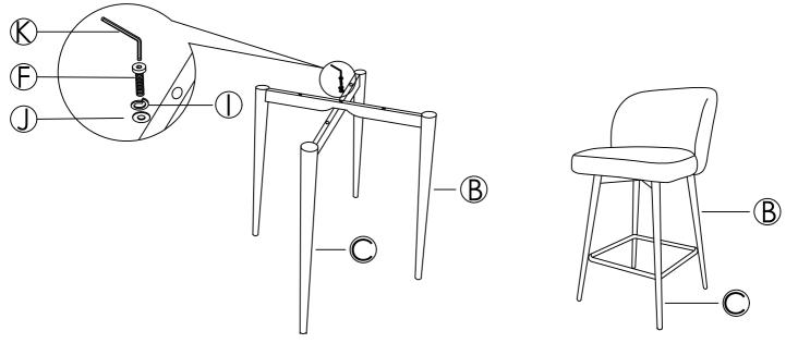
2 Loosely attach the bolts (H) one by one and keep them loose. Do not fully tighten. After loosely attach the first bolt, move on to the diagonal bolt. After all 4 bolts are attached, use allen wrench (K) to tighten. Note: Do NOT use power tools for assembly.
