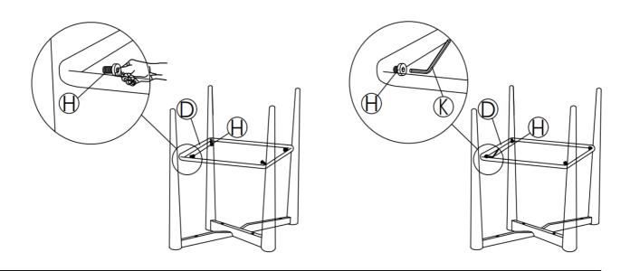
3 Fully tighten the longest bolt (F) in step 1 with allen wrench (K). Then attach swivel plate (E) to assembled legs in step 2, using longest bolts (F), lock washers (I), flat washers (J) and allen wrench (K). **Do not fully tighten yet.**
