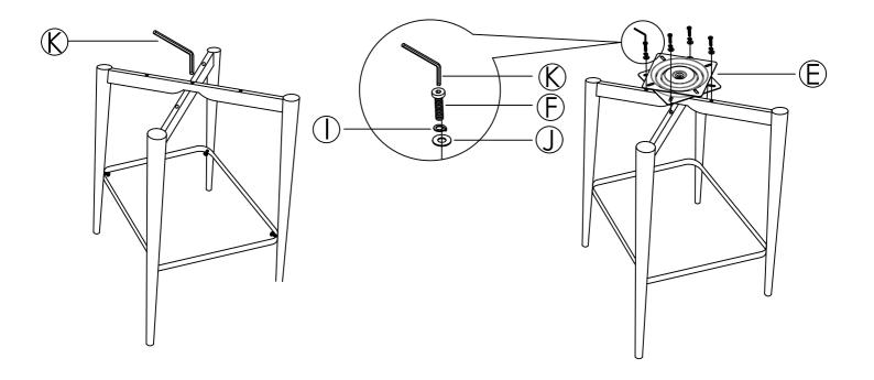
Put assembled legs in step 3 on a flat surface. Push legs up or down as necessary to level. Once level, tighten all bolts.
