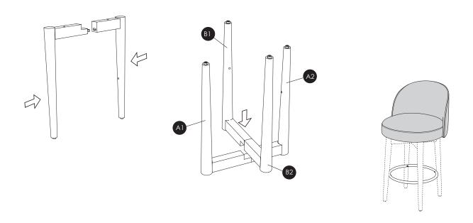
2 Attach Foot Ring (D) to assembled stool base in Step 1. Loosely attach the Bolts (H2) one by one and keep them loose. Do not fully tighten. After loosely attach the first bolt, move on to the diagonal bolt. After all 4 bolts are attached, use Allen Wrench (T2) to tighten.
