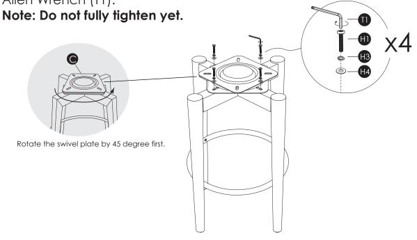
4 Put assembled stool base in Step 3 on a flat surface. Push legs up or down as necessary to level. Once level, fully tighten all bolts.
