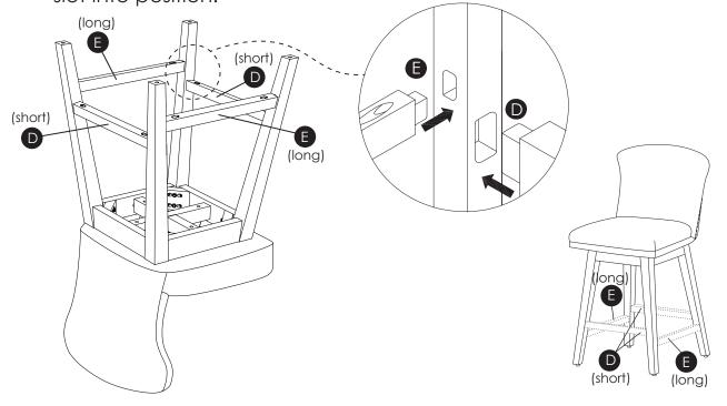
3 Attach the rails using screws (H1). Do NOT start the screws if the rails are not fully slotted into position.
