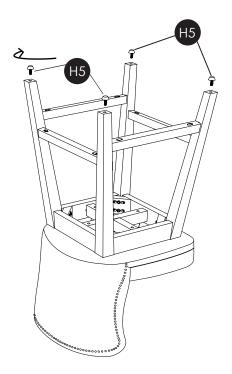
Turn assembled chair upright and place on a flat surface. Push legs up or down as necessary to level. Once level, tighten all bolts and screws. Note: Each leg has an adjustable foot leveler to help level your chair.
