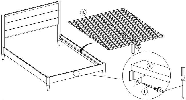
Attach assembled slats x8 (2 Set) (10) to side rail (5), using Wood Screw M4 X 30MM (J) and Phillips Head Screwdriver (Not Included). Fully tighten.
