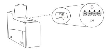
Step 1: Rotate the Legs (B) firmly, and gently place the Console in the upright position.
