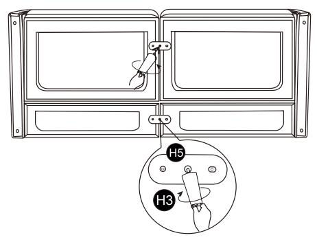
6 Slide washer (H2) into the stud of wood leg (H3). Then attach the wood leg to the bottom of left and right arms. Fully tighten.
