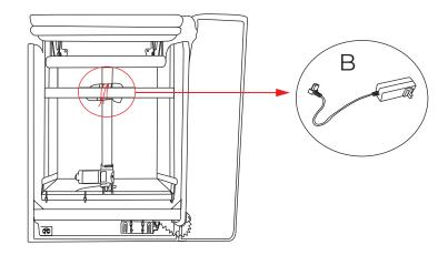
Gently place the Power Right Chair in the upright position. Connect the Power Cord (B) into the DC adaptor located at the back corner of the seat.
