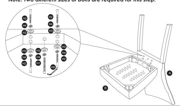
3 Attach front legs (C) to seat (B), using short bolts (H1), lock washers (H4), flat washers (H3), and allen wrench (H5).
