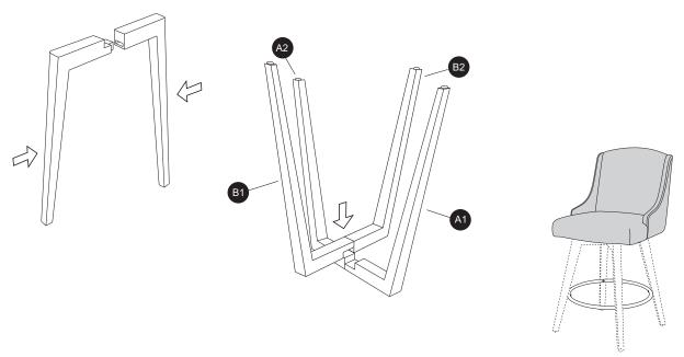
2 Flip over the stool base. Loosely attach the Bolts (H2) one by one and keep them loose. Do not fully tighten. After loosely attach the first bolt, move on to the diagonal bolt. After all 4 bolts are attached, use Allen Wrench (T1) to tighten.
