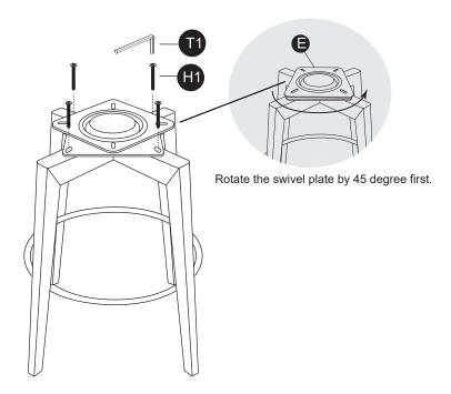
4 Put assembled stool base in Step 3 on a flat surface. Push legs up or down as necessary to level. Once level, **fully tighten all bolts.**
