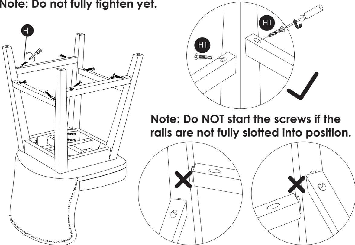
**Note: Do NOT start the screws if the rails are not fully slotted into position.**
