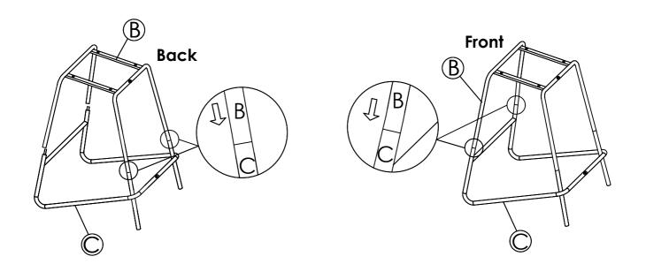
Attach upper leg (B) to lower leg (C), using shorter bolts (E), and allen wrench (H).
