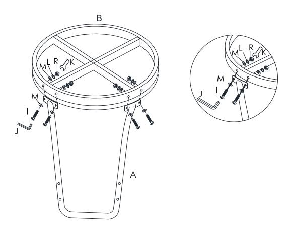
Attach Screw (G) to assembled stool seat, using Bolts (O), Spring Washers (L), and Flat Washers (M) After all 4 bolts are attached, use Allen Wrench (J) to tighten.
