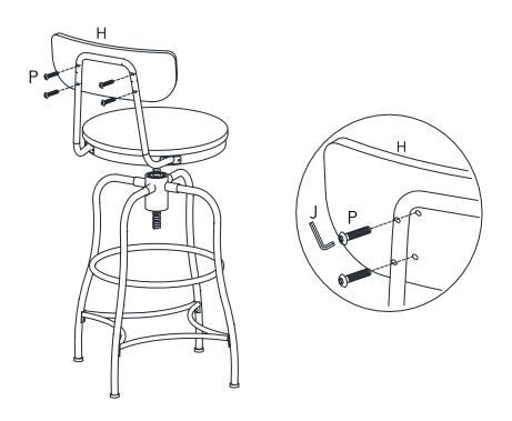
Put assembled stool on a flat surface. Push legs up or down as necessary to level. Once level, tighten all bolts.
