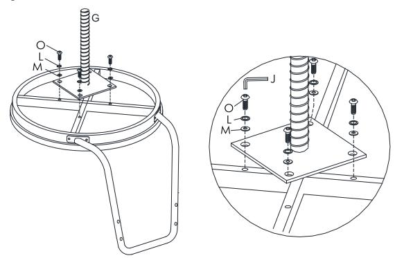
6 Slide the assembled stool base into Screw (G). Attach Bolt (O) to Screw (G). Use Allen Wrench (J)to tighten.
