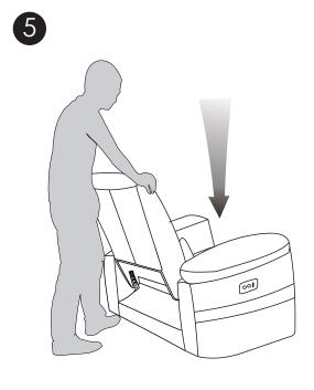
Push down firmly on seat back to lock connector.
