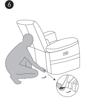
Affix back cover to bottom of the frame using the built-in hook and loop fastener strip.
