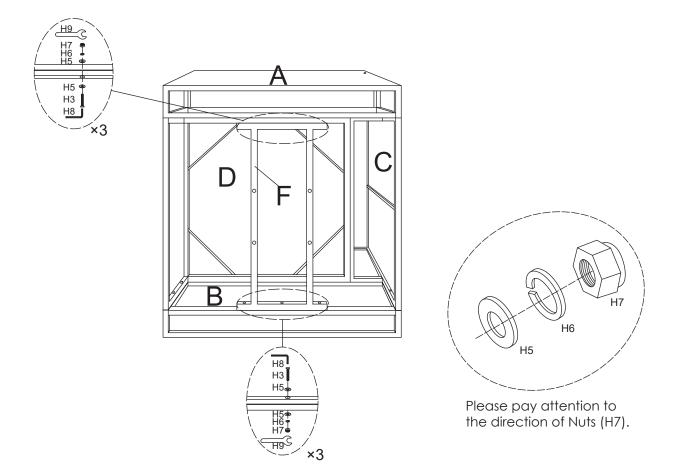
Attach Metal Ring (E) to the assembled part in previous step, using Bolts (H2), Flat Washers (H5), Spring Washers (H6), Nuts (H7), Allen Wrench (H8), and Open-Ended Wrench (H9). Use the Open-Ended Wrench (H9) to hold the Nuts (H7) steady, use the Allen Wrench (H8) to tighten the Bolts (H2). Fully tighten.
