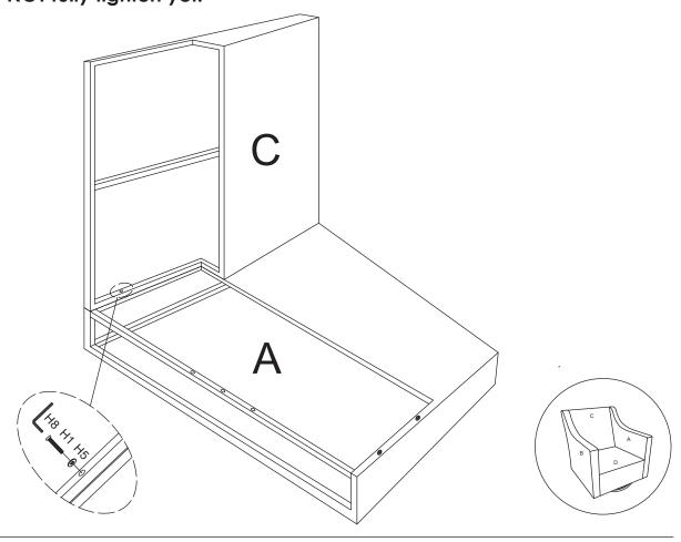
First, attach the front side of Seat Panel (D) to Right Arm (A), using Bolts (H1), Flat Washers (H5), and Allen Wrench (H8). **Do NOT fully tighten yet.**Then, attach the back side of Seat Panel (D) to Back Panel (C), using Bolts (H2), Flat Washers (H5), and Allen Wrench (H8). **Do NOT fully tighten yet.**
