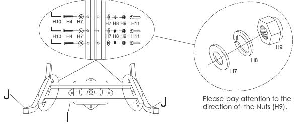
Attach Connecting Rods (H) to the assembled part in previous step, using Bolts (H3), Flat Washers (H7), Spring Washers (H8), Nuts (H9), Allen Wrench (H10), and Open-Ended Wrench (H11). Use the Open-Ended Wrench (H11) to hold the Nuts (H9) steady, use the Allen Wrench (H10) to tighten the Bolts (H3). **Fully tighten**.
