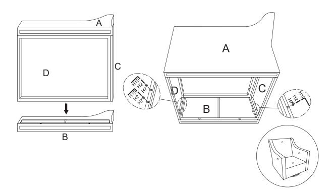
8 Place the chair upright. Attach Left Arm (B) to Back Panel (C), using Bolts (H5), Flat Washers (H7), and Allen Wrench (H10). **Do NOT fully tighten yet.**
