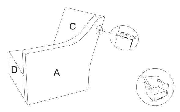
Place the Left Arm (B) flat on the floor. Attach the front side of Seat Panel (D) to Left Arm (B), using Bolts (H2), Flat Washers (H7), and Allen Wrench (H10). Do NOT fully tighten yet. Attach Back Panel (C) to Left Arm (B), using Bolts (H2), Flat Washers (H7), and Allen Wrench (H10). Do NOT fully tighten yet.
