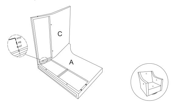
5 First, attach the front side of Seat Panel (D) to Right Arm (A), using Bolts (H2), Flat Washers (H7), and Allen Wrench (H10). **Do NOT fully tighten yet.**
