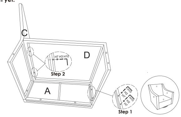
6 Place the chair upright. Attach Right Arm (A) to Back Panel (C), using Bolts (H5), Flat Washers (H7), and Allen Wrench (H10). **Do NOT fully tighten yet.**
