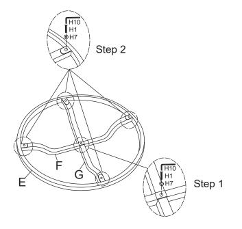
Attach the assembled metal base to the swivel plate, using Bolts (H2), Flat Washers (H7), Spring Washers (H8), Nuts (H9), Allen Wrench (H10), and Open-Ended Wrench (H11). Use the Open-Ended Wrench (H11) to hold the Nuts (H9) steady, then use the Allen Wrench (H10) to tighten the Bolts (H2). Fully tighten.
