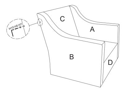
9 Set the button on Ratchet Wrench (H12) at "-". Use Ratchet Wrench (H12) to fully tighten all bolts in Step 4, 5, 6, 7, and 8.
