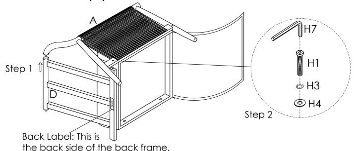
Attach Right Arm (B) to Seat (C), using Big Flat Washers (H5), Lock Washers (H3), Short Bolts (H1), and Allen Wrench (H7). **Do not fully**
