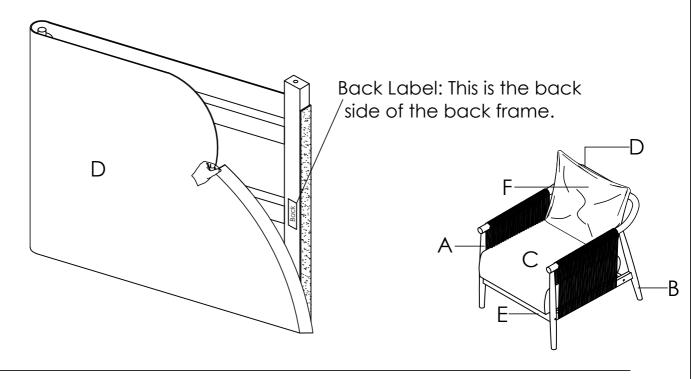
Attach the upper side of Back Frame (D) to the upper side of Left Arm (A) as indicated below (Step 1). Attach the bottom side of the Back Frame (D) to the bottom side of Left Arm (A), using Small Flat Washers (H4), Lock Washers (H3), Short Bolts (H1), and Allen Wrench (H7), as indicated below (Step 2). **Do not fully tighten yet.**
