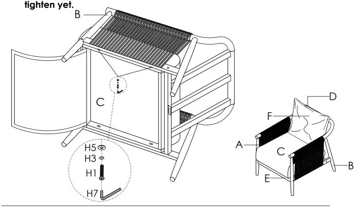
Attach Right Arm (B) to Back Frame (D), using Small Flat Washers (H4), Lock Washers (H3), Short Bolts (H1), and Allen Wrench (H7). **Do not fully tighten yet.**
