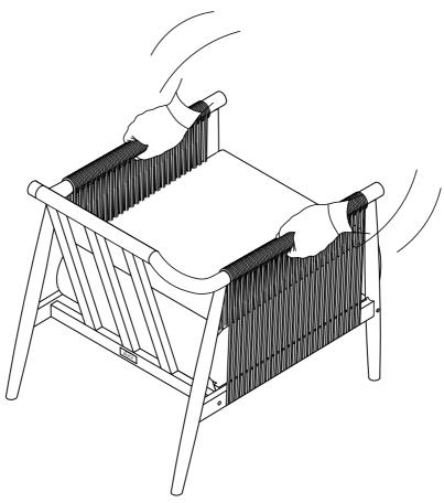
Fully tighten all bolts in Step 2, 3, 5, 6, and 7 (Eight bolts in total). Attach the Velcro underneath the Seat (C) as indicated below.
