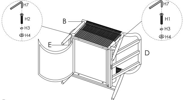
Attach Back Frame (D) to Left Arm (A) and Right Arm (B), using Flat Head Screw (H6) and Allen Wrench (H7). Fully tighten.
