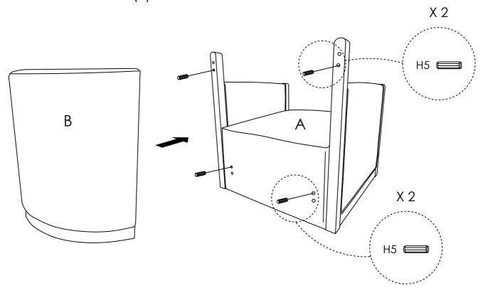
2 Move on to the holes from Backrest (B), use Lock Washers (H3), Long Bolts (H2) and Allen Wrench (H6) to assemble. **Do not fully tighten yet.**
