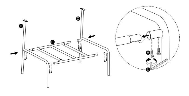
2 Attach Metal Back Bracket (A) to assembled metal base in Step 1, using Bolt (H) and Allen Wrench (L). Note: Do not fully tighten bolts.
